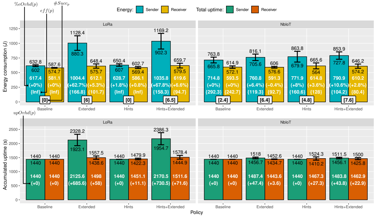
Fig. 3. Simulation results for 1 minutes uptime (average of 200 seeds with standard deviations as error bars). The upper bar charts display energy metrics, the other the uptime metrics. Each energy bar charts has four values: (i) the average energy consumption, (ii) eOvhd(p) in parenthesis, (iii) eff(p) in curly brackets and (iv) \#Succ_p in square brackets. For the uptime bar charts, two values are shown: (i) accumulated uptime and (ii) upOvhd(p) in parenthesis.
